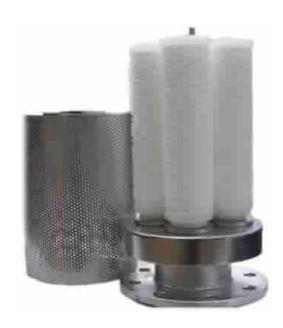
Flowrite "TB" Series Tank breather filters are fabricated from 304-Stainless Steel. They are designed for a maximum operating pressure of 100 kPa at 80°C, depending on cartridges fitted. The "TB" Series housings feature Flowrite's well proven centre post and nut design.
